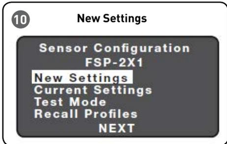
New Settings allow you to select the different sensor parameters such as: High/Low mode, Time Delay, Cut Off, Sensitivity, Setpoint, Ramp/Fade rates and Photocell. See **Figure 10**.
